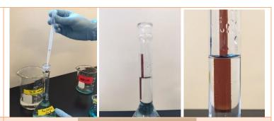
Place stopper on volumetric flask. Holding stopper tightly in place, gently invert the flask to mix well.
