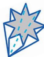
Figure 7. Open fluted (or fan-folded) filter paper
