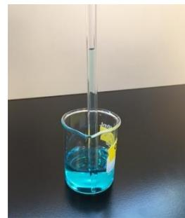
Remove the pipet bulb and quickly use your index finger to seal the top of the pipet.
