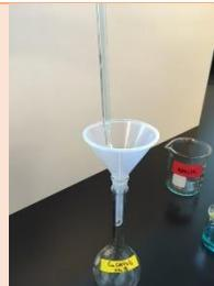
Again, touch the pipet tip to the side of the receiving flask to transfer any drop left hanging.
