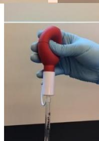
Place the tip of the pipet in the liquid.
