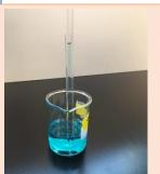
Remove the pipet bulb and quickly use your index finger to seal the top of the pipet. Turn the pipet on its side and rotate it as you change its angle to rinse the inside walls of the pipet with the solution. Transfer the solution in the pipet into the waste beaker. Repeat this process at least one more time. Don't forget to dry the outside of the pipet before placing it inside the solution.
