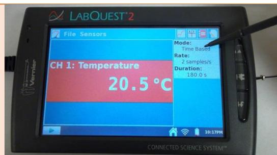
Adjust "Interval" and "Duration" per experiment's instruction. If not stated in experiment, ask your instructor. (ignore Rate). Then press "OK". [Note - these do not stay in memory. Before starting each new run you must reenter the Interval and Duration values.]
