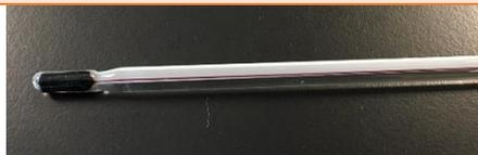
Place the thermometer in the sample. Make sure that the bulb portion is submerged in the sample, and that it is not touching the walls or base of the container.
