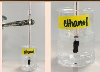
Once the reading has stabilized, read and record the measurement to the proper number of significant figures.
