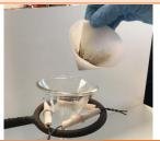
The solid on the filter paper is called the residue. The aqueous portion is now called the filtrate. Follow the experiment's instructions regarding the residue and the filtrate.
