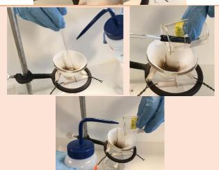
Once the aqueous portion has filtered, rinse the solid with your wash bottle. Allow the liquid to drain. Then rinse one or two more times, allowing the liquid to drain between rinses.
